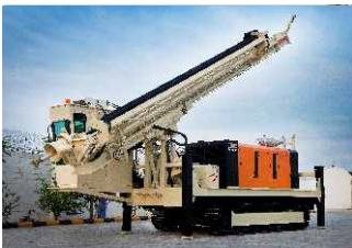
Blast hole drilling
