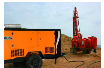
High pressure compressor for crawler drilling
